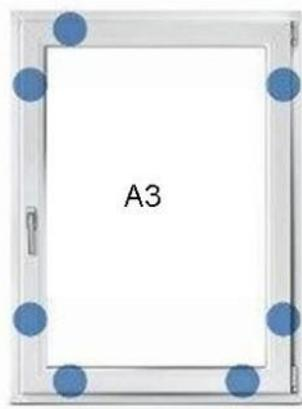
The Fauser wood window and door system uses exclusively **Tilt & Turn** opening mechanism: a 90 degree turn of the handle opens the window like a casement, for easy egress/regress and also for easy cleaning. Another 90 degree turn of the handle will tilt the window inside on top. This allows for ventilation while still providing security and also keeping the rain out.
